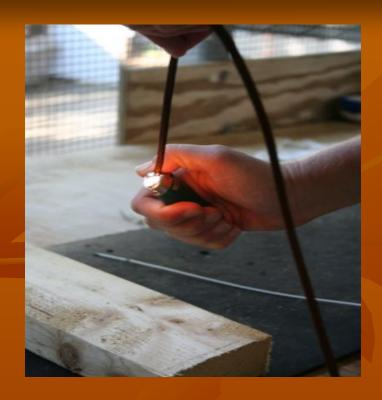
Light one end of your parachute cord. Let the cord catch on fire, then immediately blow the flame out and let the end come to a blunt point and cool. (Caution, the burnt end of the parachute cord is very hot!)
