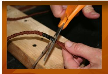
\_ Once the braid is sealed cut off excess cord right up to the edge of the melted braid and discard
