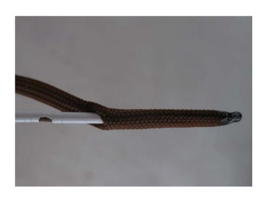
Next, take the previously burnt end of the cord and measure roughly 3 inches below that end. On the back side of the cord (the side opposite of the hole that was just made in the center of the cord), insert the wire coat hanger. Once again, being careful not to go through the other side of the cord. Push the hanger inside of the cord until the point of the hanger reaches the burnt end of the cord.
